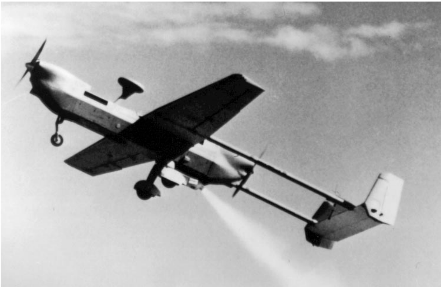
Figure 1: Hunter UAV: Wingspan 29' Length 23'
