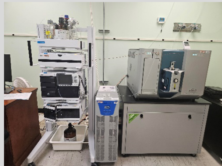
FSIS Eastern Laboratory mass spectrometer and SCIEX 7500, used to test samples and detect compounds.
