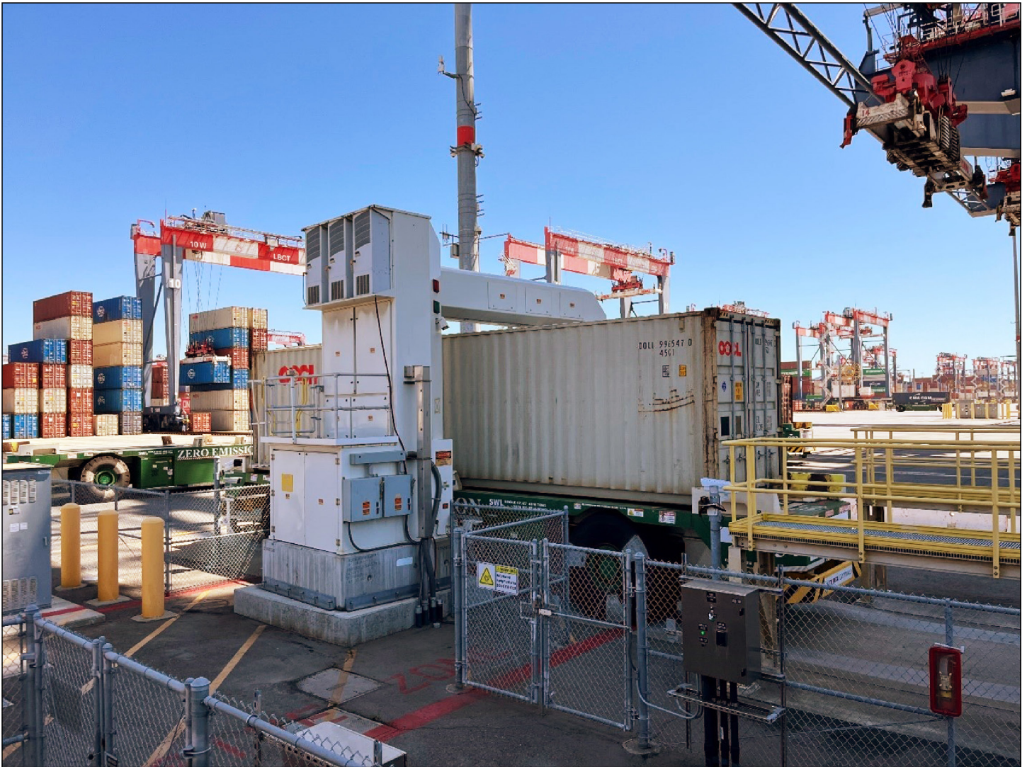
Figure 8: A Shipping Container Passing Through U.S. Customs and Border Protection’s Non-Intrusive Inspection Screening Equipment at the Long Beach Container Terminal Within the Port of Long Beach
