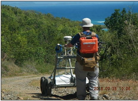
Figure 9: Advanced Geophysical Classification Technology Used at Cleanup Sites on Vieques and Culebra, Puerto Rico
