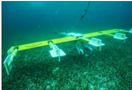
Detection of potential munitions is done by measuring and recording magnetic anomalies caused by the presence of iron objects lying on or beneath the seafloor.
