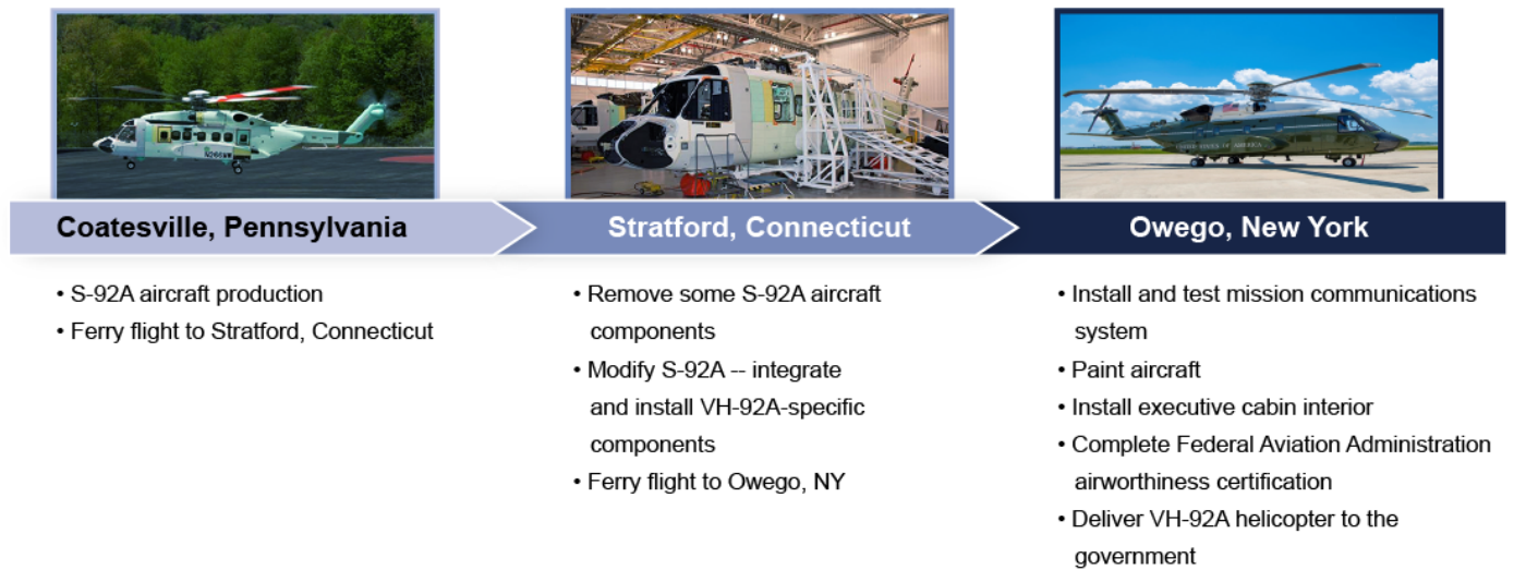
Figure 1: Modification of the S-92A Commercial Helicopter to the VH-92A
