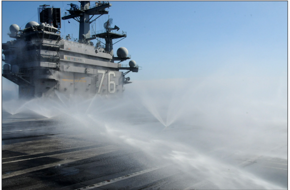
Figure 9: Demonstration of Countermeasure Wash Down System on the USS Ronald Reagan Aircraft Carrier
