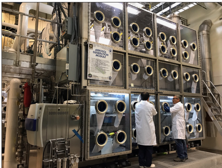
Figure 8: Researchers Preparing Particle Analyzer for Calibration in the Whole System Live Agent Test Chamber at the BioTesting Division, Dugway Proving Ground, Utah
