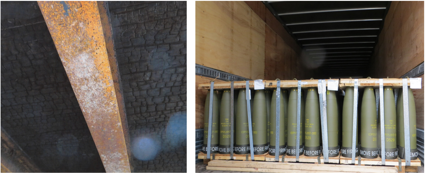
Figure 10: Burned Underside of TPS Carrier's Trailer after Fire Incident and Undetonated High Explosives inside Trailer.
