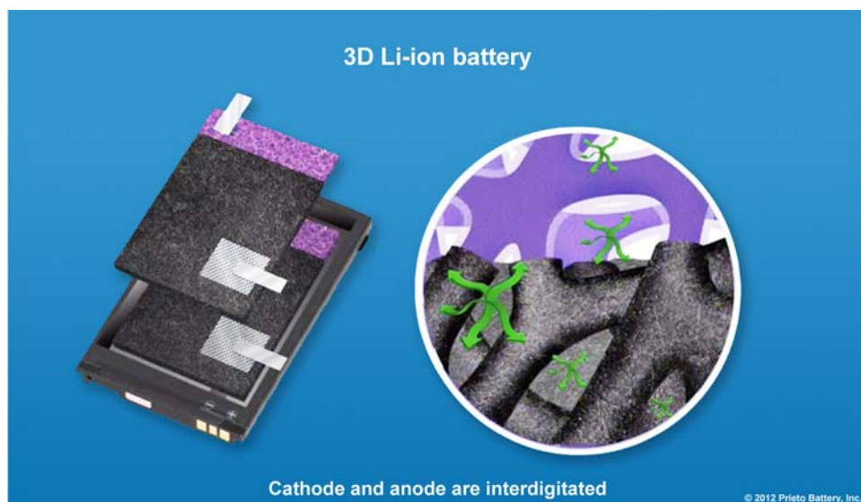
Figure 10: Illustration of a 3D Lithium-Ion (Li-ion) Battery
