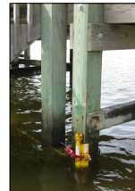
Figure 3: U.S. Geological Survey (USGS) Storm Tide Sensor Deployed Prior to Hurricane Irene
