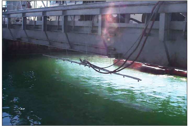
Spray bar applying dispersant to oil in tank.
