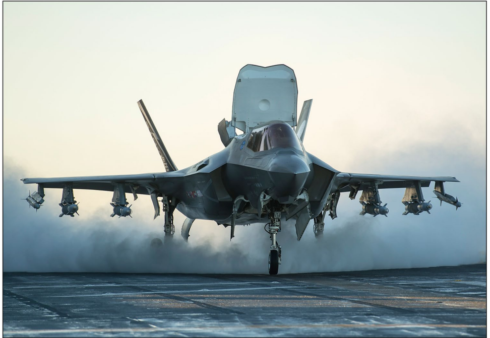
Figure 1: An F-35B Exercising Its Short Takeoff and Vertical Landing Capability on the USS America
