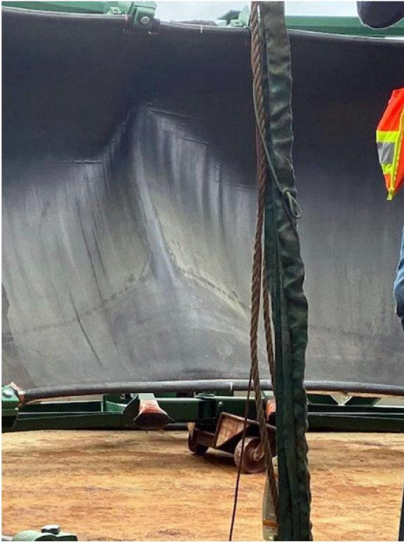
Figure 10: Damaged Rubber Window of Sonar Dome
