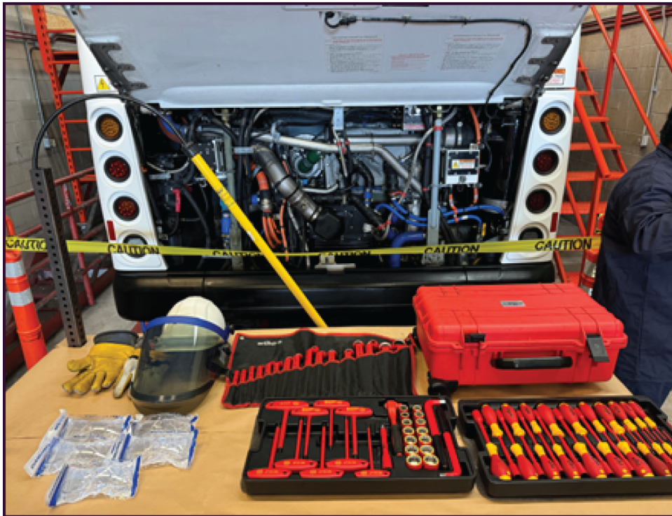
Figure 6: Personal Protective Equipment and Other Tools Used by Mechanics Who Maintain Zero-Emission Buses
