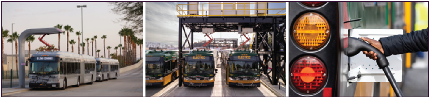
Figure 1: Examples of Charging Infrastructure for Battery Electric Bus Propulsion Include En-Route Chargers, Overhead Charging Stations, and Plug-In Chargers
