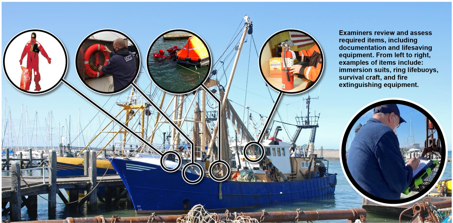
Figure 2: Examples of Items a U.S. Coast Guard Examiner Reviews during a Dockside Exam
