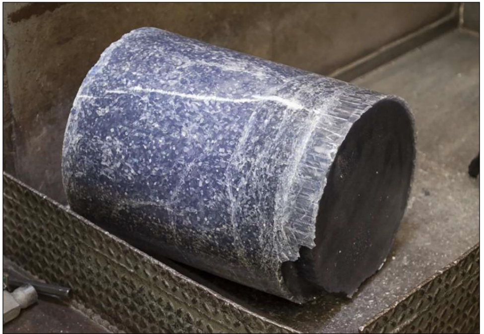
Figure 2: Lithium Feedstock Before Crushing into Powder and Machining to Produce Nuclear Weapons Parts
