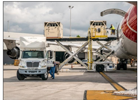
Figure 1: Air Cargo Pallet and Cargo Loaded onto an Aircraft
