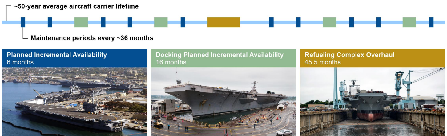
Figure 2: 36-Month Aircraft Carrier Maintenance Cycle over the 50-Year Expected Service Life
