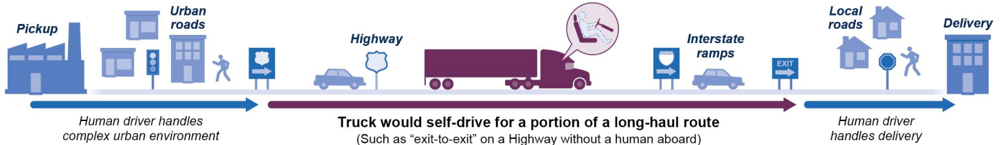
Figure 4: Illustration of Commercial Truck Self-Driving for Part of a Long-Haul Route
