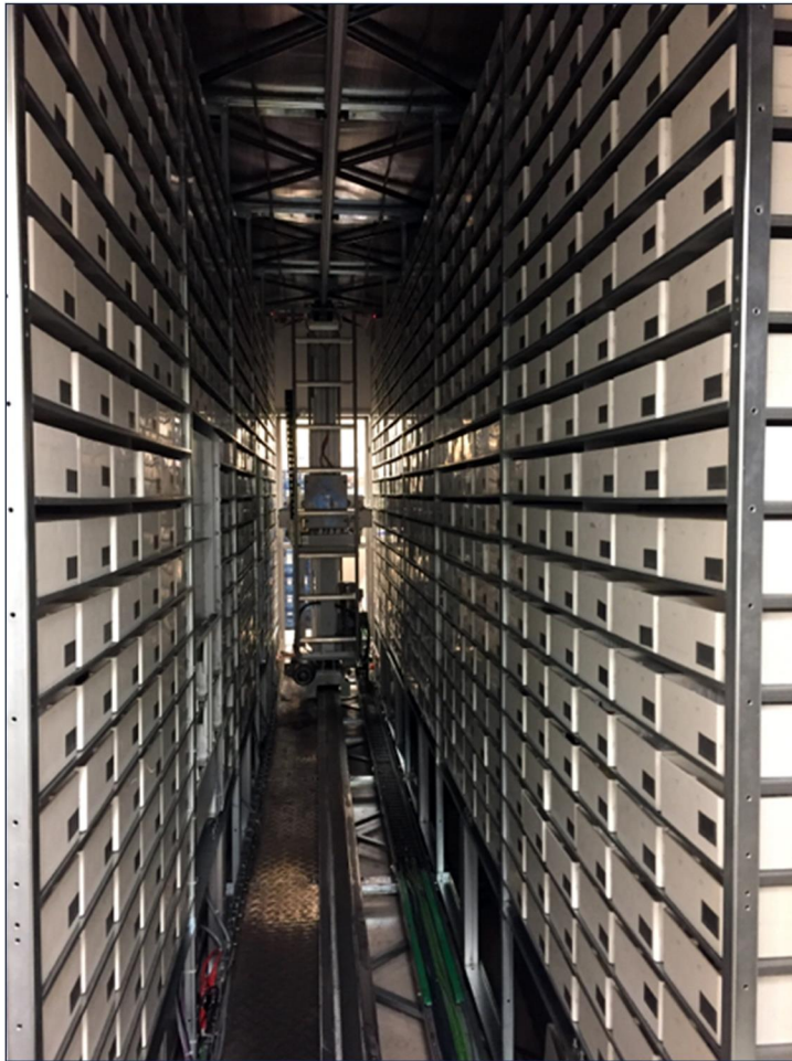
Figure 3: Automated Medication Dispensing Machine at a Department of Veterans Affairs Medical Center
