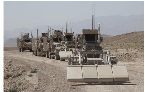
The photographs above depict a warfighter using a handheld device to detect improvised explosive devices (IED) (left) and vehicle enhancements to detect and disable IEDs (right).
