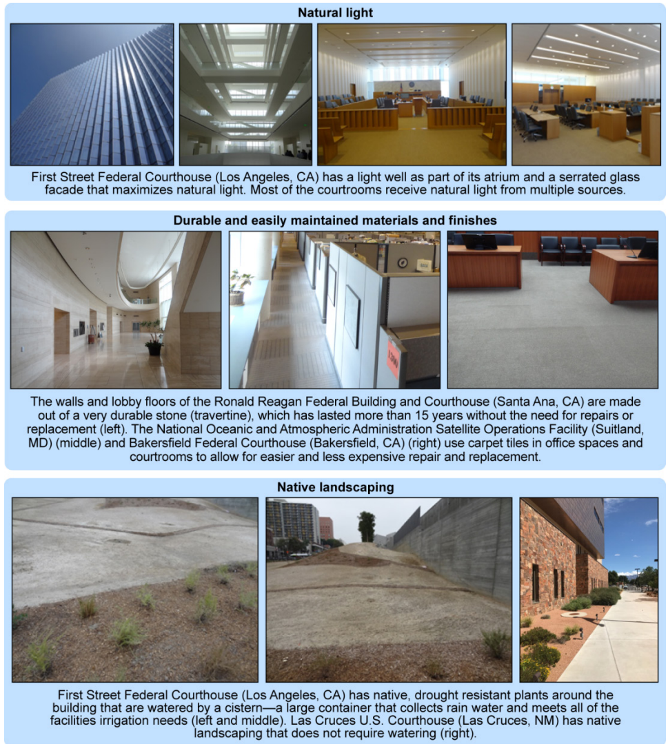
Figure 2: Design Excellence Buildings with Durable and Easily Maintained Materials and Finishes, Low Maintenance Landscaping, and Increased Natural Light, according to Building Managers
