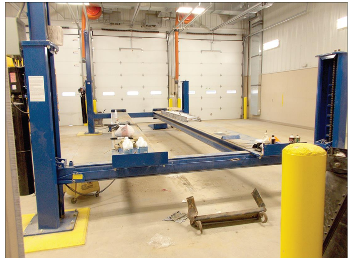
Figure 7: Exterior and Interior of Recently-Constructed School Bus Maintenance Building Where Door Does Not Close When a Large School Bus Is On Hydraulic Lift
