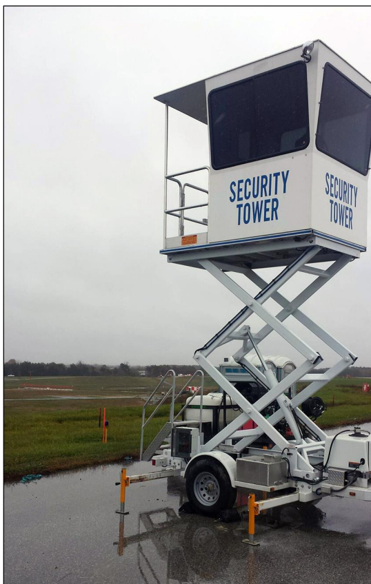
Figure 4: Mobile Surveillance Tower at a Commercial Airport
