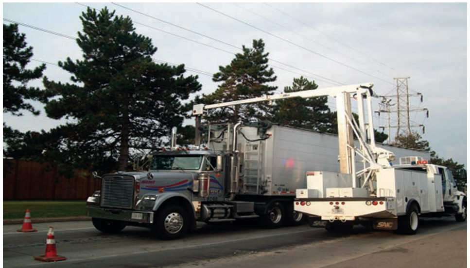
Figure 11: Mobile VACIS Scanning Shipment in Secondary Inspection
