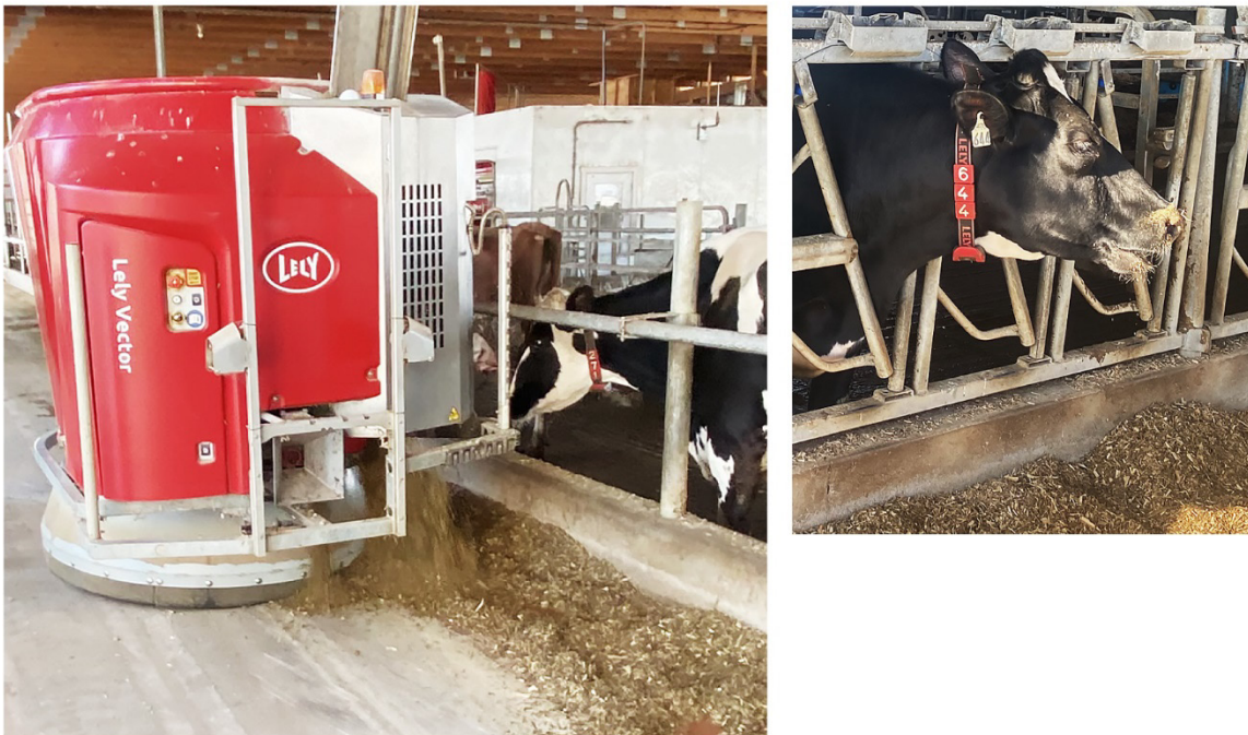
Figure 3: Autonomous feed delivery robot and activity monitor
