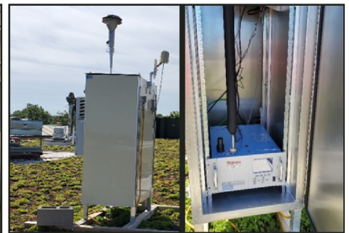
Particulate matter monitoring site atop a building at the Illinois State Fairgrounds operated by the Illinois Environmental Protection Agency
