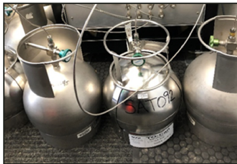
Canisters used to collect samples for measuring air toxics operated by the Wisconsin Department of Natural Resources
