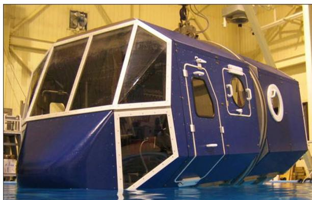
Egress simulators simulate the interior and exterior of a helicopter and are used to teach students how to exit a crashed and submerged helicopter. They can be configured differently to simulate different kinds of helicopters by changing where the seats are placed as well as the types of windows and doors used on the simulator.
