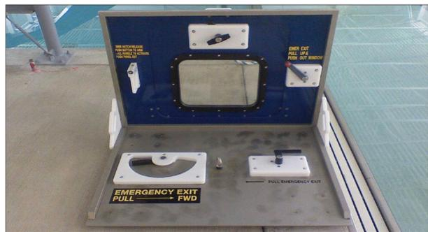
A Shallow Water Initial Memory Mechanical Exit Release device, a type of problem-solving trainer used by the Navy to teach students to operate helicopter exit release controls underwater and develop their confidence prior to training in its egress simulators.
