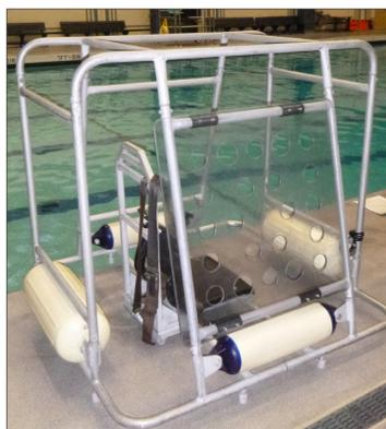
Egress trainers simulate the interior of a helicopter—including an exit, seatbelt, and window—so that students can practice the steps involved in exiting a submerged helicopter.
