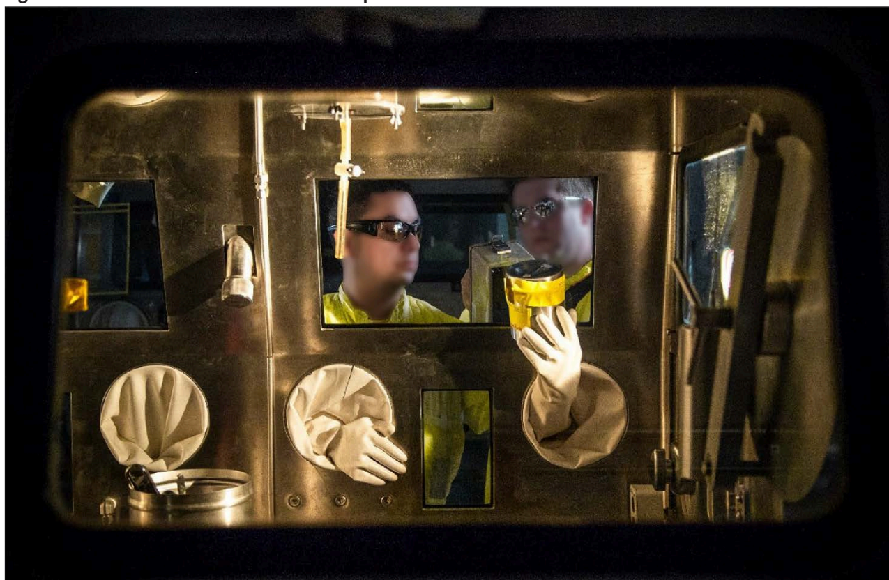
Figure 27: Sealed Glovebox for Plutonium Operations
