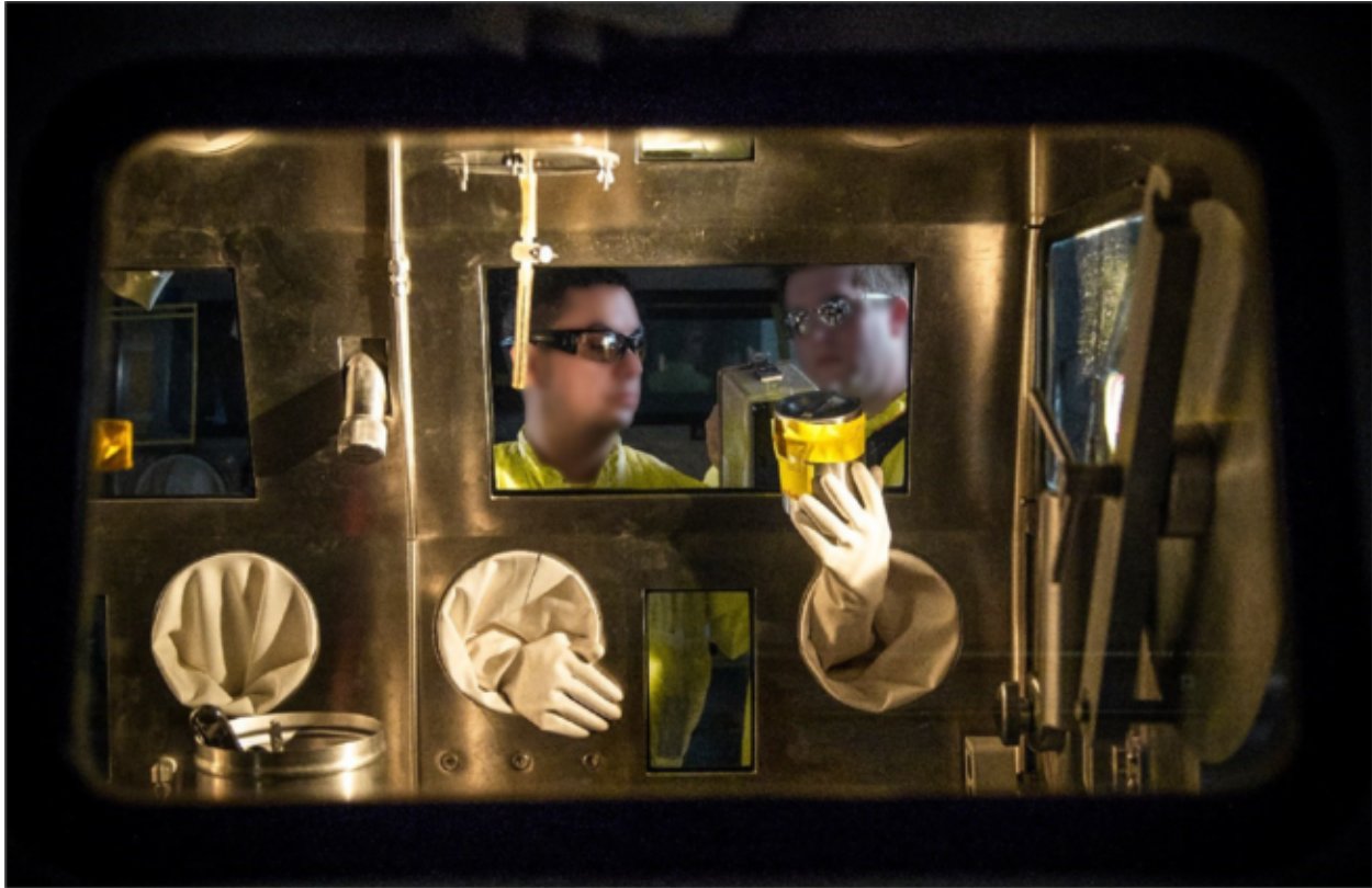
Figure 27: Sealed Glovebox for Plutonium Operations
